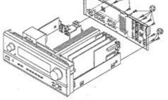
(1) Remove 12 screws ⑬, 1 screw ⑭, and 4 screws
